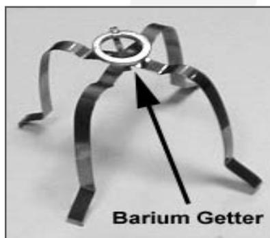
The Getter is located at the bottom of the outer tube.
